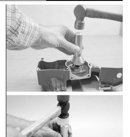
20.15 Install crankshaft into clutch side of case.
